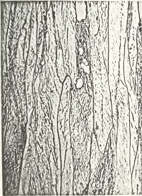
FIG. 29 AT 482°C FOR 1.5 HOURS (ROCKWELL 30T 66.9)
